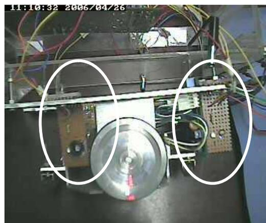
Figure 7: Infra-Red Sensor Module
