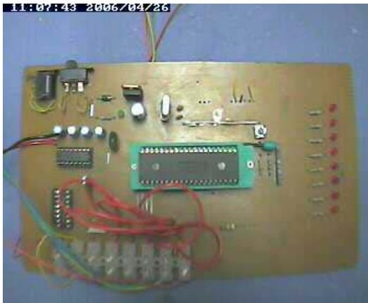
Figure 12: RS 232 Compatible PIC 16F877A Demonstration Board
